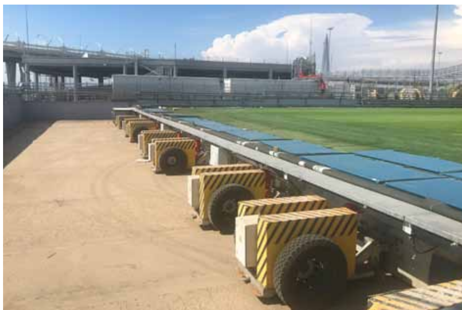
Electric motors to move the pitch in and out of the stadium
